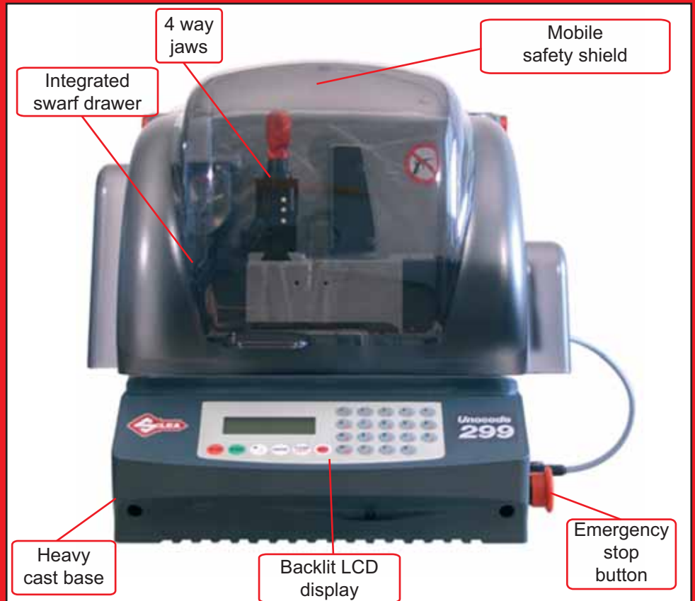
UNOCODE 299 Cylinder code key cutting machine.
